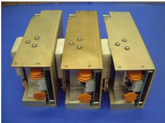
*Fig (5b) 3 Isolated output PFC made of 3 modules. This combination will connect to Delta input of 115V line to line and deliver one 250VDC output to 3KW*
