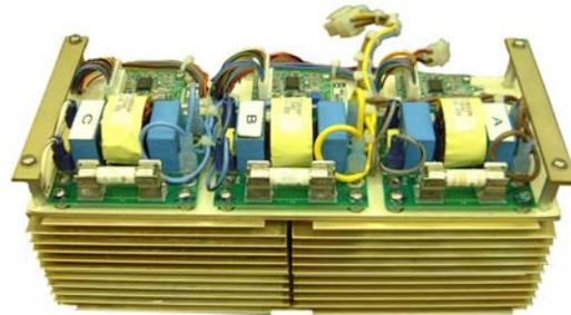
Fig (3b) One block of 3 non-isolated PFC modules can deliver 250VDC up to 3KW. Was tested up to 4.5KW output.
