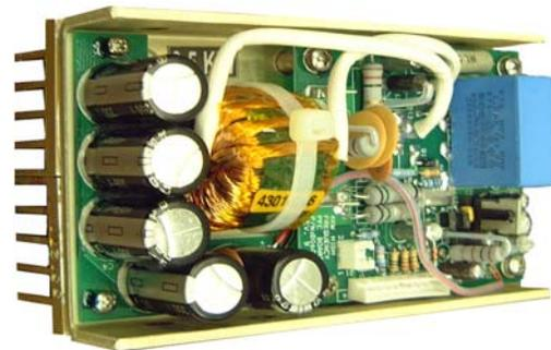
Fig.(3a) Single non isolated PFC Module accepts and delivers 250VDC 1KW. 130-170Vrms.
