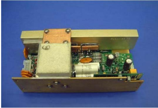
*Fig (5a) Single isolated PFC module delivers 1KW output from line to line voltage. The isolated output is 250VDC*
